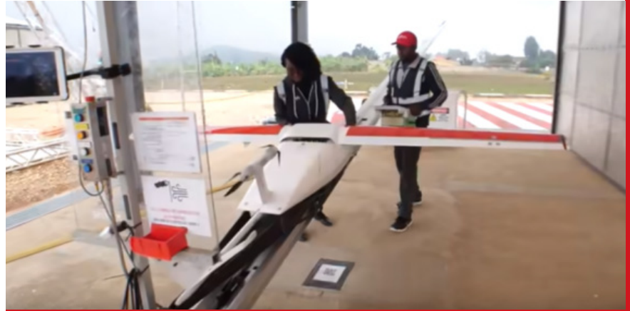
Photo: Open Source Photography Workers prepare a Zipline drone for a delivery by installing the wings and battery pack.
