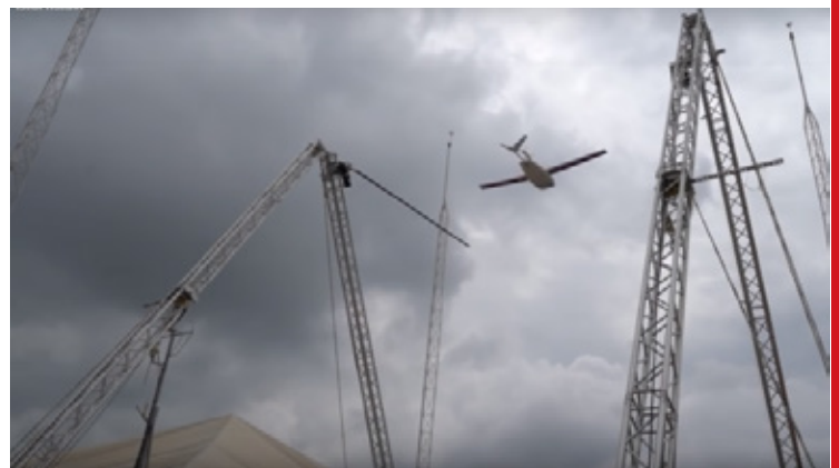
Photo: Open Source Photography A Zipline drone prepares to engage its small tail hook onto catch line and swing nose down to make a “landing”.
