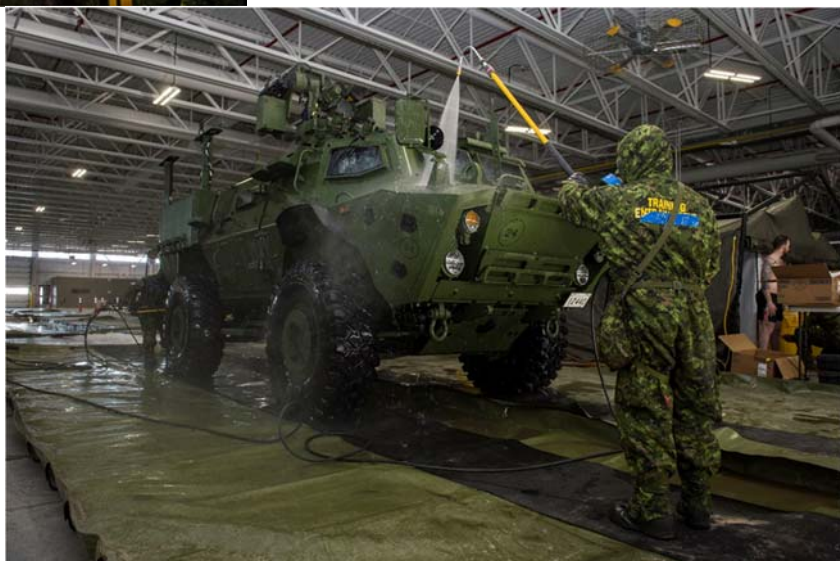
A 2 Svc Bn Decontamination Operator spraying DF200 decontaminant on a Tactical Armoured Personnel Vehicle (TAPV) to eliminate the CBRN hazard.
